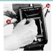
1. Open the back cover and pull out the upper spool change knob (31), then insert an empty spool into the take-up spool chamber (36) so that it engages the winding axis. Let go of the spool change knob.
